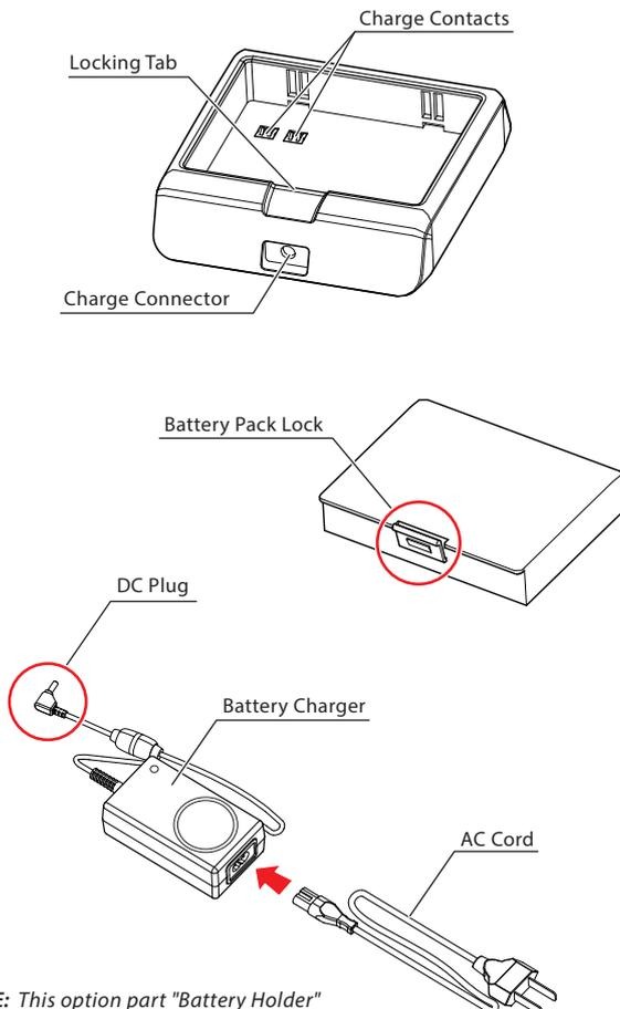
**NOTE:** This option part "Battery Holder" does NOT include the battery charger.
