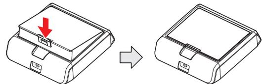
2. To recharge the battery, install the battery pack in the Battery Holder T300. Insert the DC Plug into the charge connector and plug the AC Cord into a power outlet.
